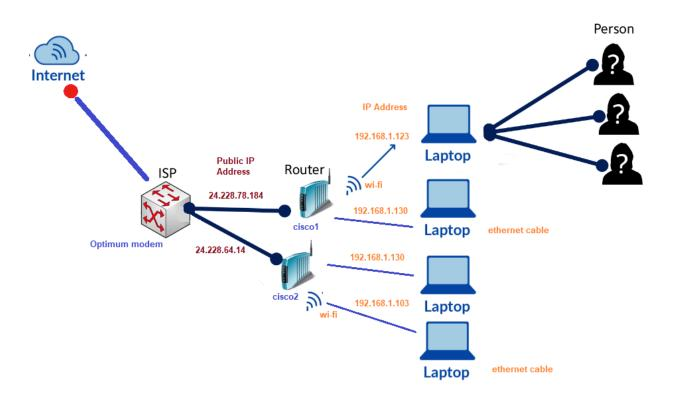
When you connect your PC by a cable to the router (or modem) of the Internet provider, you have an ethernet connection. Otherwise, you would be connected wireless.
